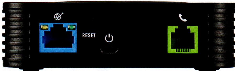
Grandstream's HandyTone HT801 VoIP adapter has two ports on the back – one for Ethernet (blue), one for your phone (green)
